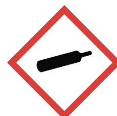
Gas under Pressure
